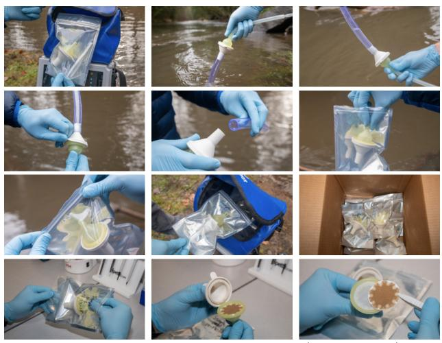
Note: Self-preserving filter housings are currently rated to 10 PSI max pressure (20 in.-Hg; 508 mm-Hg). Please program your eDNA Sampler for a 10 PSI pressure threshold.
