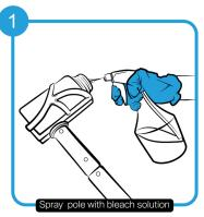
Spray the part of the sampling pole that touched the water with bleach/water solution
