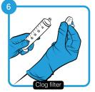
Remove filter and repeat steps 3, 4, 5 & 6 until filter is clogged
