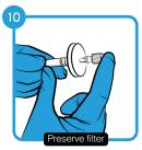
Place preservative cap onto the other end of the filter to seal the sample
